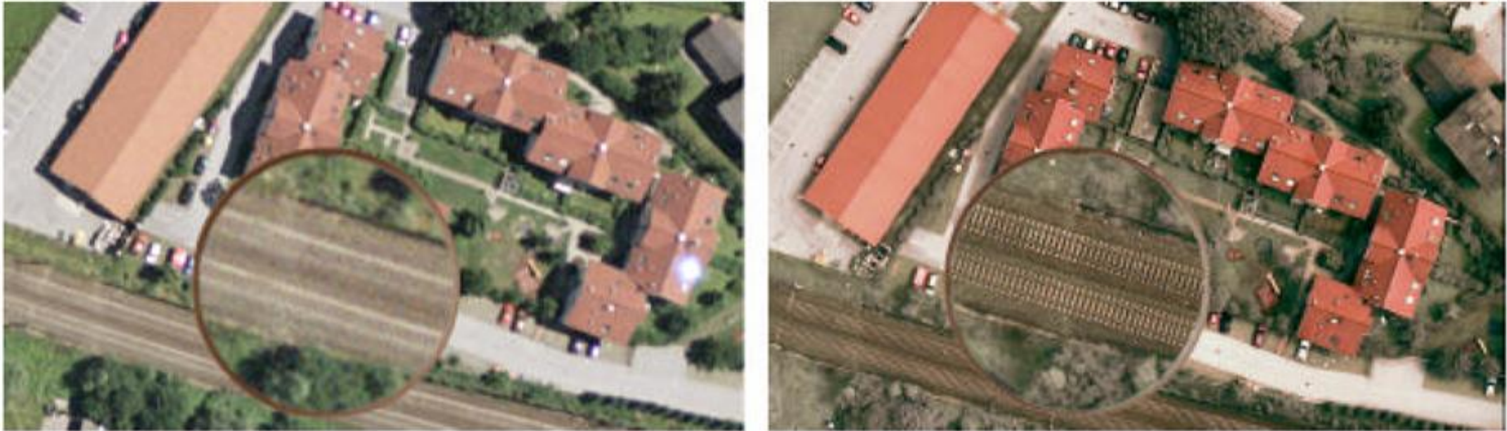
Figure 6: Color image segment from aerial film (left) with a GSD of 15 cm, obtained from a 12.5\mu\text{m} scan. The UltraCam-image has a GSD of 16 cm (right). The inserts are 2x enlarged and have a diameter of 150 pixels. Note the definition of the railroad track.
