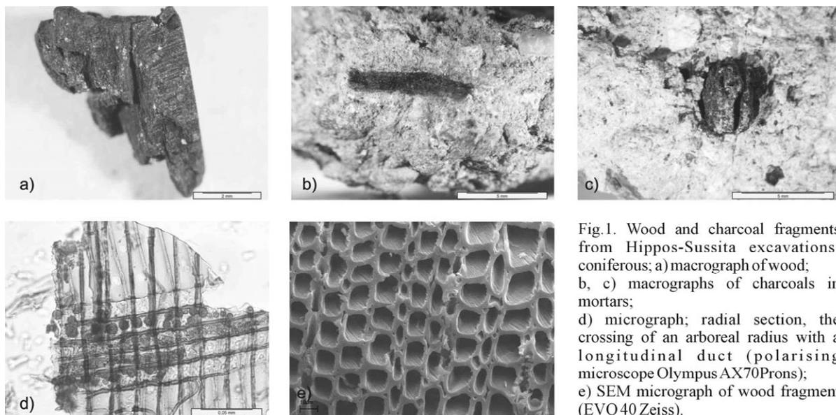
Fig.1. Wood and charcoal fragments from Hippos-Sussita excavations; coniferous; a) macrograph of wood; b, c) macrographs of charcoals in mortars; d) micrograph; radial section, the crossing of an arboreal radius with a longitudinal duct (polarising microscope Olympus AX70Prons); e) SEM micrograph of wood fragment (EVO 40 Zeiss).
