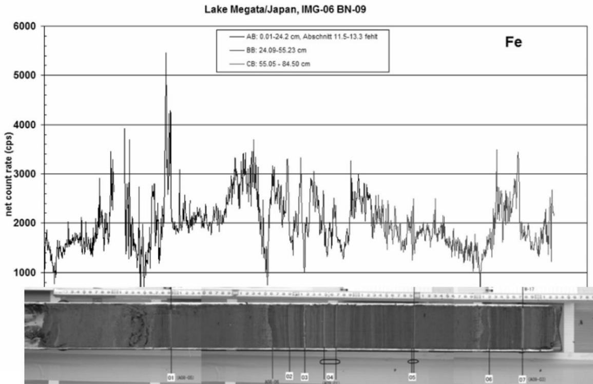
Fig 1: Varved lacustrine sediments of Lake Ichi-no-Megata core BN09 (depth 605–685 cm). Graph shows high resolution X-ray-fluorescence variations in chemical composition (here for iron) characterising the varves, turbidites, and tephra-layer sediments in comparison to the core (photo).
